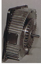
Fig.1 Thruster with axial air gap and disk rotor.
