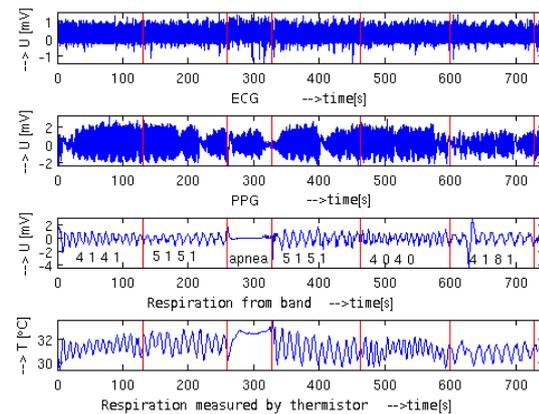
Fig. 1. Signals that were measured during controlled respiration. Patterns were changing continually after 2minutes. The apnea phase duration was about 62s.
