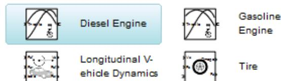
The Vehicle Components library contains blocks that represent components of a full vehicle beyond the drivetrain itself. It includes models of engines, wheeled vehicles, and tires in contact with the ground. The blocks of this library serve as suggestions for
