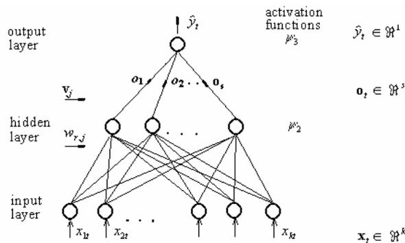
Figure 4: Fully connected single hidden layer network
