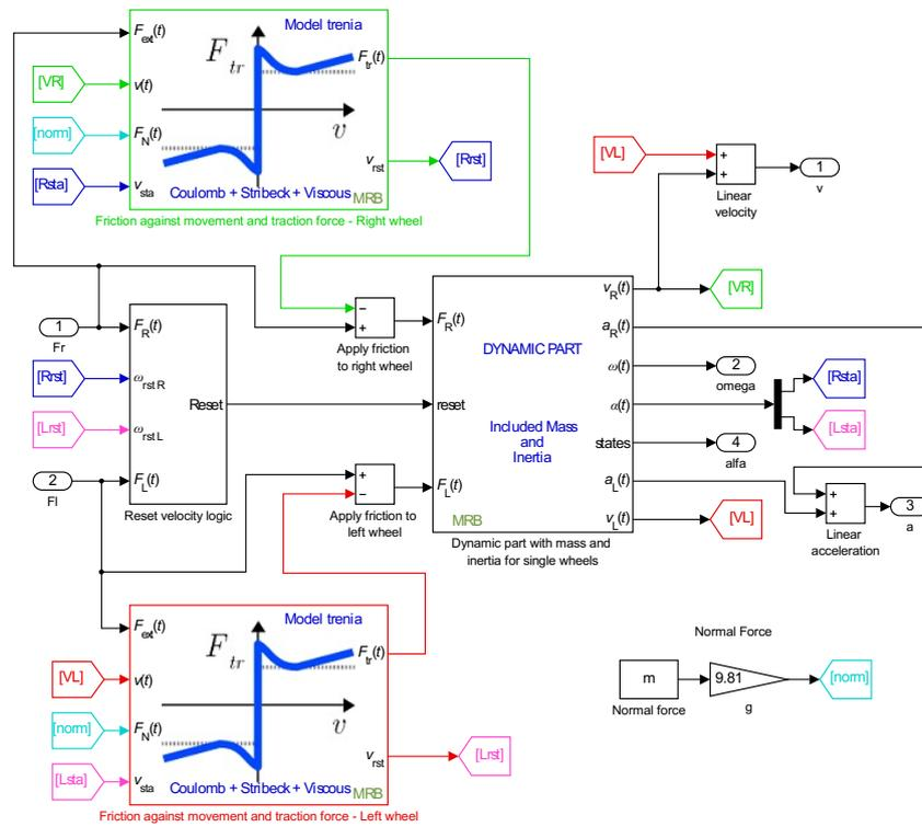
Figure 7: Dynamic model of the mobile robot extended by adjustable friction
