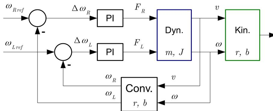
Figure 13: Diagram of a mobile robot with an internal control loop
