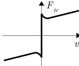
Figure 5: Generalized model of friction - a function of velocity  $v$
