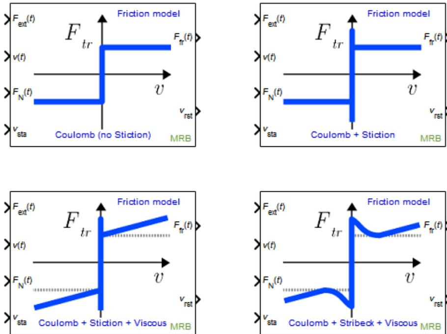
Figure 6: Different setting for created friction model in Simulink
