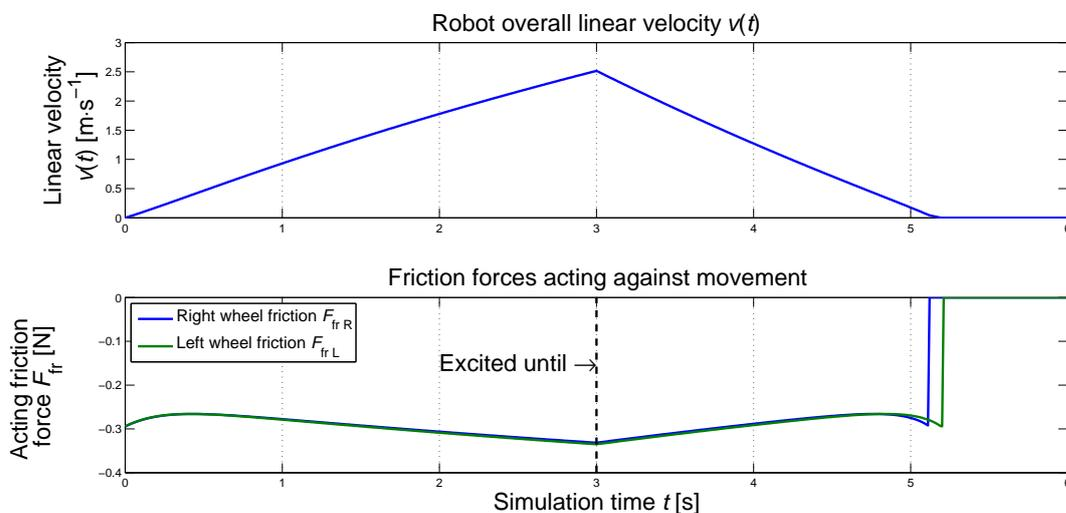
Figure 11: The simulation experiment - the overall linear velocity and the impact of friction forces to the robot wheels
