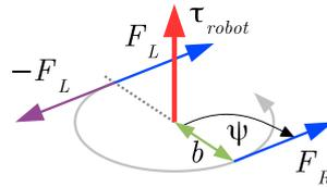
Figure 2: Definition of mobile robot's overall torque  $\tau_{robot}$  and orientation of traction forces  $F_R, F_L$
