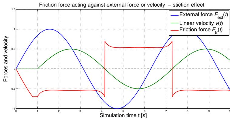
Figure 9: The generalized friction - the effects of static and kinetic friction with regard to the external force and caused linear velocity
