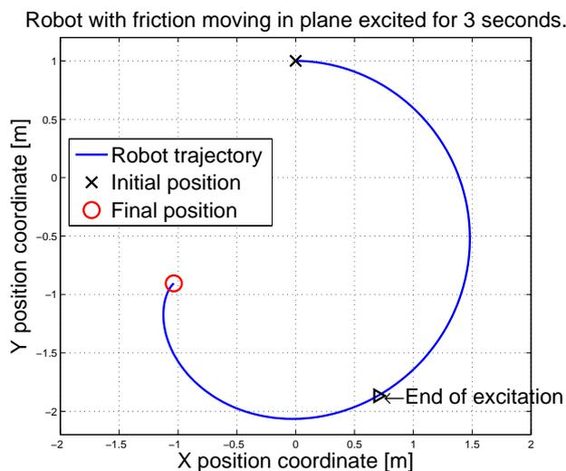
Figure 12: The simulation experiment - robot movement in the plane affected by friction
