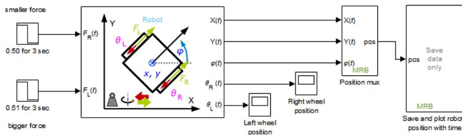
Figure 10: The simulation experiment for demonstration of the friction effects acting on mobile robot movement
