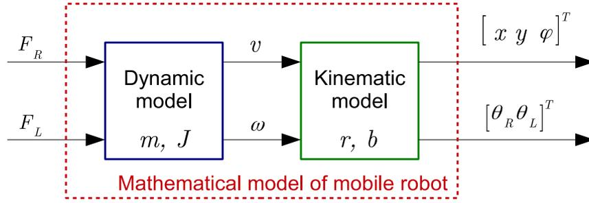
Figure 3: Block diagram of a mobile robot with the wheel engines traction forces as inputs and the position coordinates as outputs
