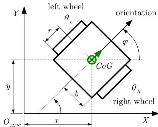
Figure 1: Definition of mobile robot dimensions and position in global coordinate system
