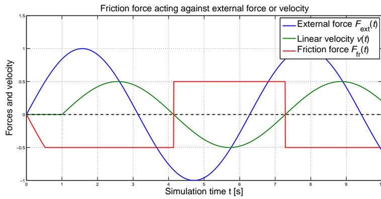
Figure 8: The Coulomb friction - effects of static and kinetic friction with regard to the external force and caused linear velocity
