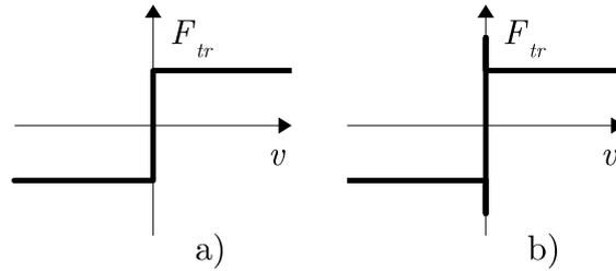
Figure 4: Friction models: a) Coulomb friction model, b) Coulomb friction model with stiction effect
