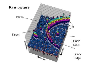
• The output of FFT for each individual sweep represents input data to RDP processing
