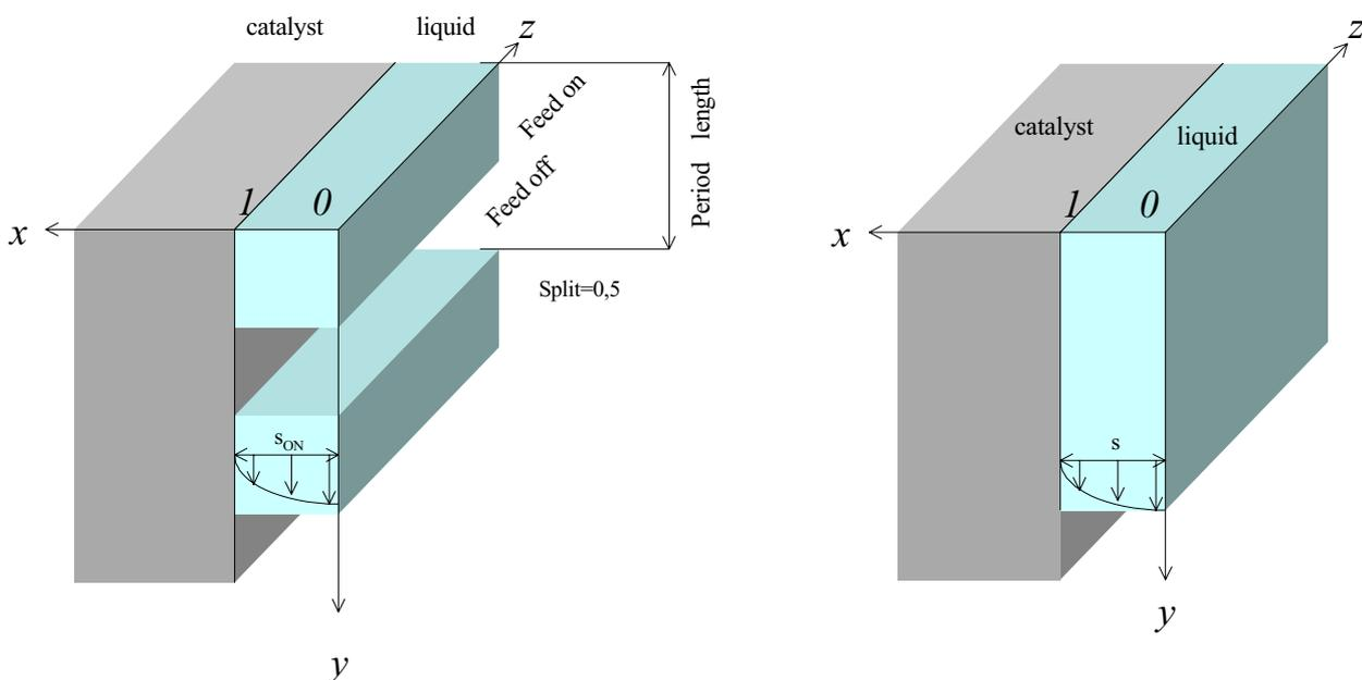
The steady state and pseudo-steady state models, for isothermal regime of reactor, were formulated and solved in this study. The liquid flow was assumed to be a laminar one. Numerical simulations were made for a simple, irreversible, monomolecular, first order
