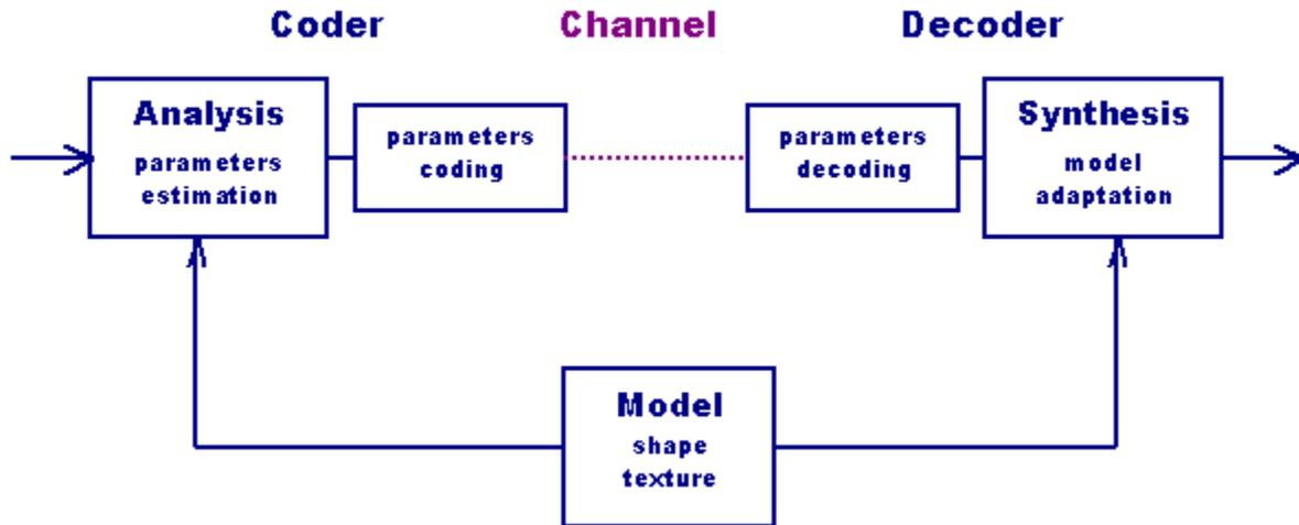
Fig. 1. System for image coding based on models
