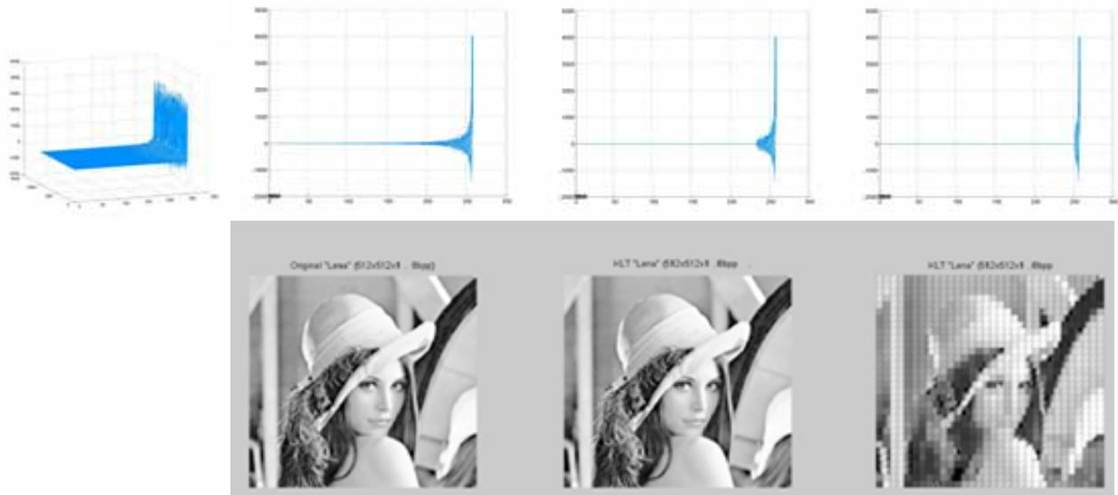
Fig. 2. Image „Lena“ coded with KLT block size 16x16, a/ KLT spectrum matrix, b/ Spectrum matrix – side view, c/ 80% of near zero coefficients zeroed, d/ 99,96% of near zero coefficients zeroed with relation to reconstructed image
