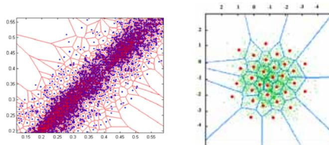
Fig.4. Voronoi diagram with assigned centroids and Voronoi diagram with finished LBG algorithm iterations
