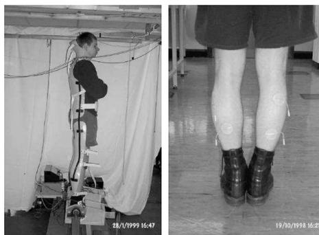
Figure 2: Subject standing in Wobbler and placement of electrodes on the calf muscle.
