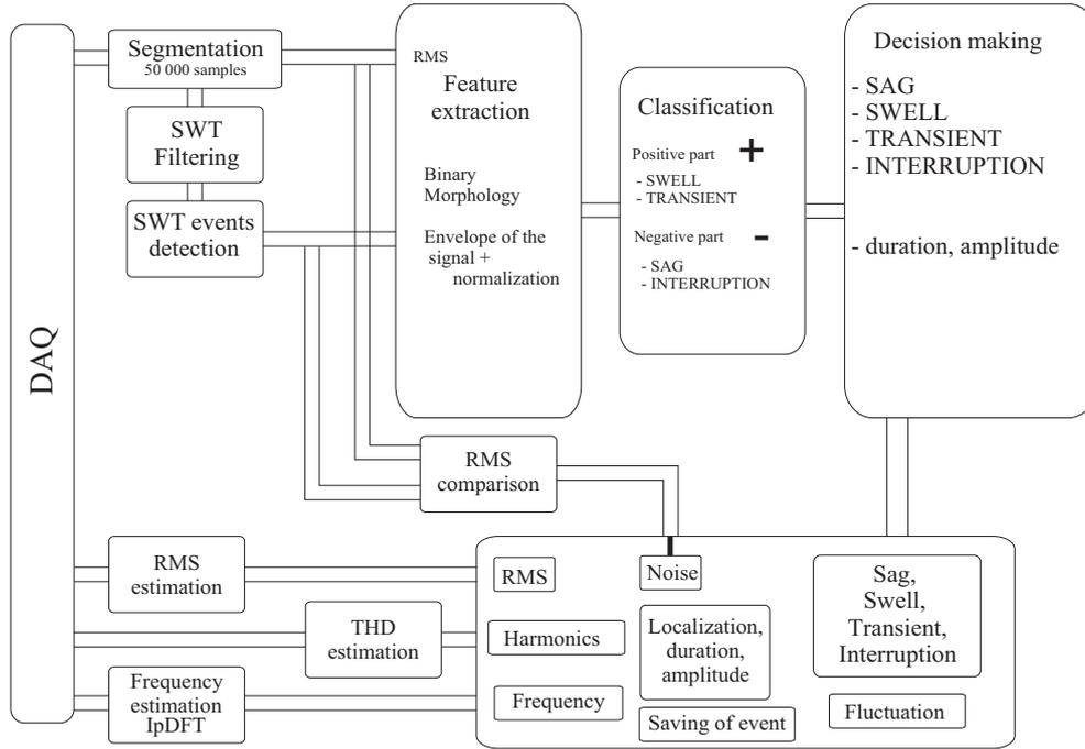
Figure 1: PQ monitoring system block diagram
