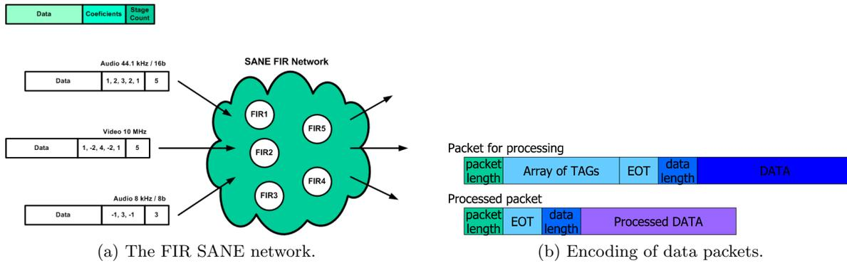
Figure 3: The FIR SANE network. Encoding of data packets.
