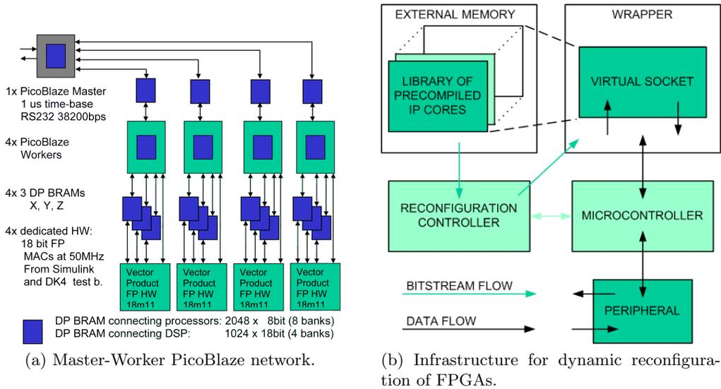
Figure 2: Master-Worker platform. Infrastructure for dynamic reconfiguration.
