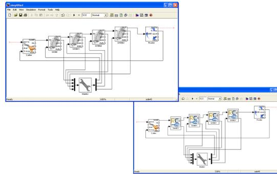
Figure 8: SANE model, simplified view, SW model (top left) and hardware in the loop (bottom right).
