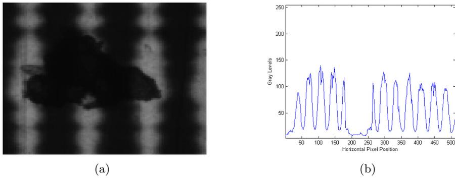
**Figure 1:** (a) Dirt Blotch on a Film Positive (b) Corresponding Gray Levels Across the Track
