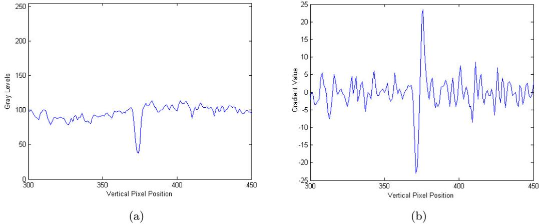
**Figure 4:** (a) Gray Levels in Column Affected by Transversal Scratch (b) Gradient of the Same Column
