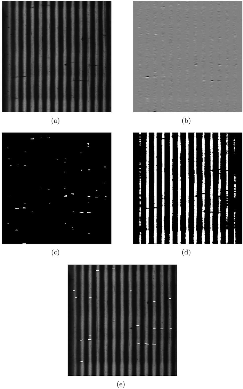
**Figure 7:** (a) Original Heavily Scratched Track (b) Gradient in Vertical Direction (c) Binary Mask before Filtering (d) Binarized Track (e) Track with Marked Scratches
