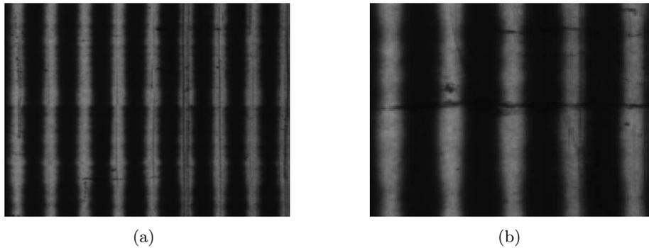
**Figure 2:** (a) Longitudinal Scratches (b) Transversal Scratches
