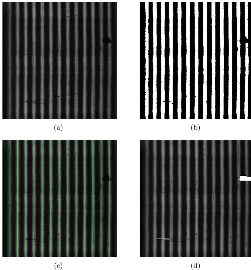
**Figure 5:** (a) Original Track (b) Binarized Track (c) Detected Traces Centers (d) Track with all Faults Marked
