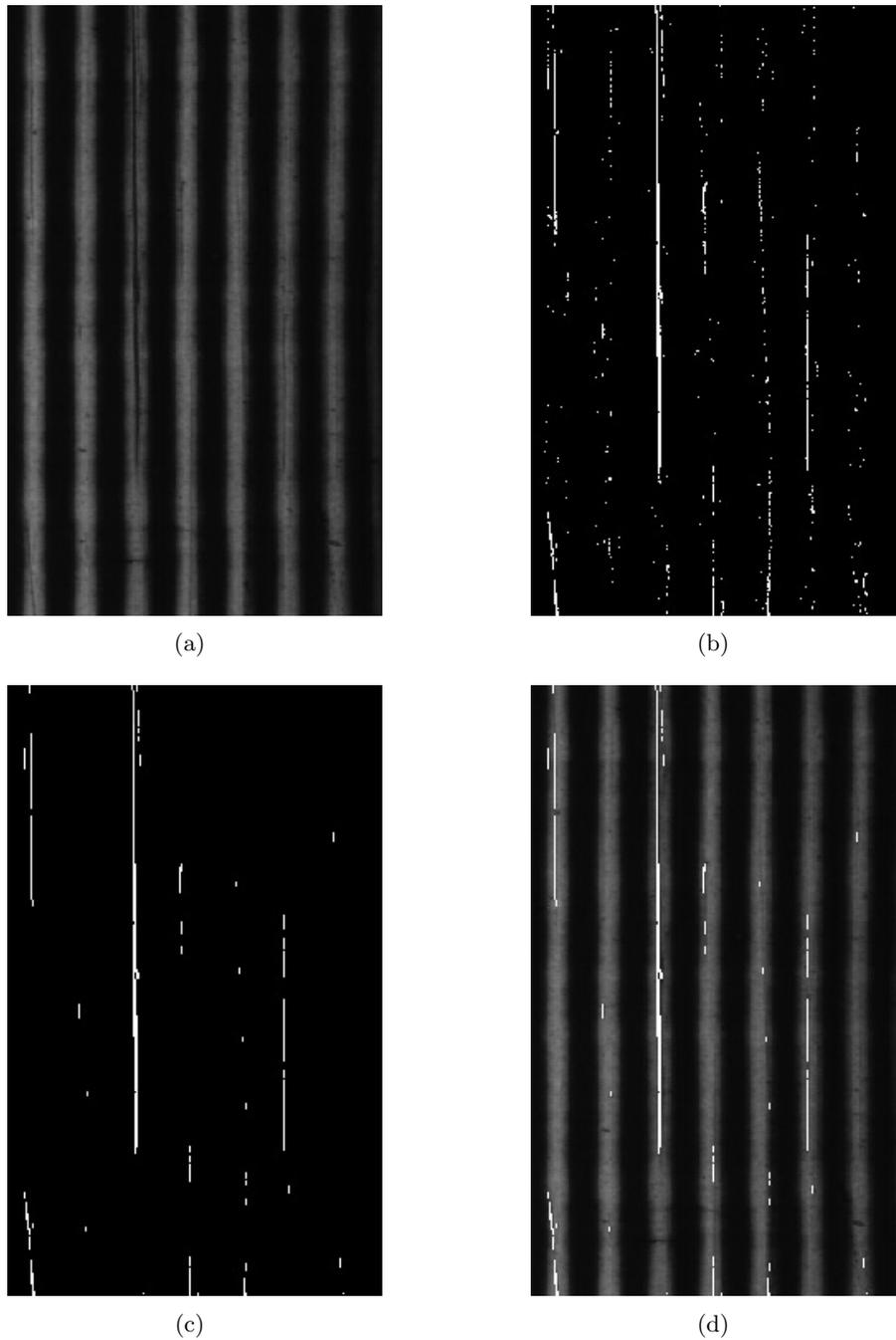
**Figure 6:** (a) Original Heavily Scratched Track (b) Binary Mask of Detected Scratches (c) Binary Mask without Faulty Detections (d) Original Track with Marked Scratches
