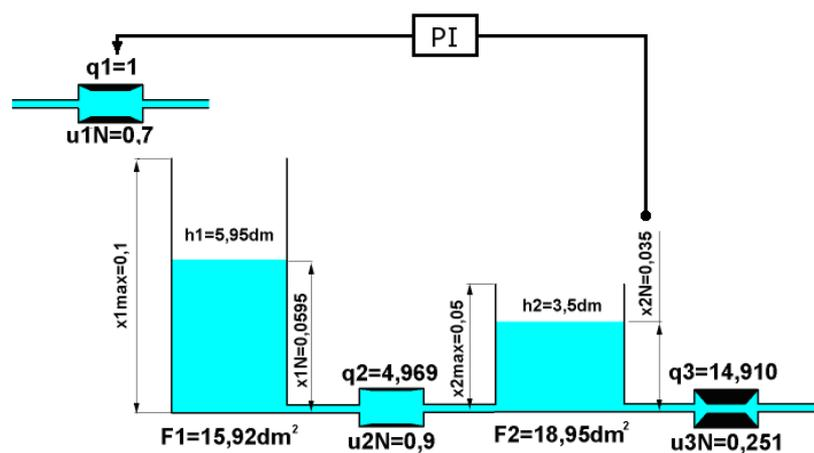
Figure 1: Two tank system with PI controller
