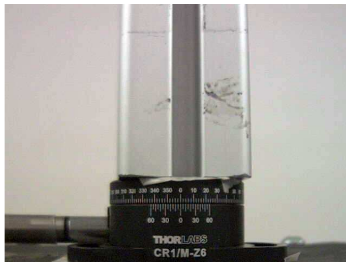
Figure 8: An aluminium profile on the rotation stage.
