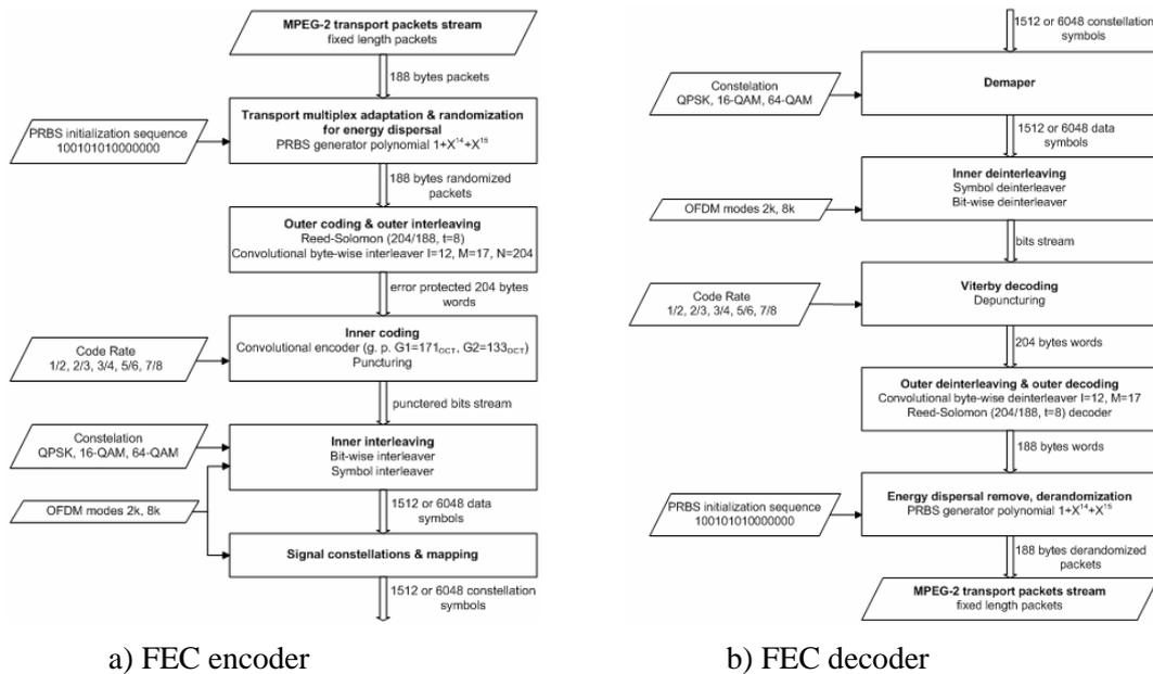
Figure 1: Flow-chart of channel coding and decoding in DVB-T (implemented in Matlab)
