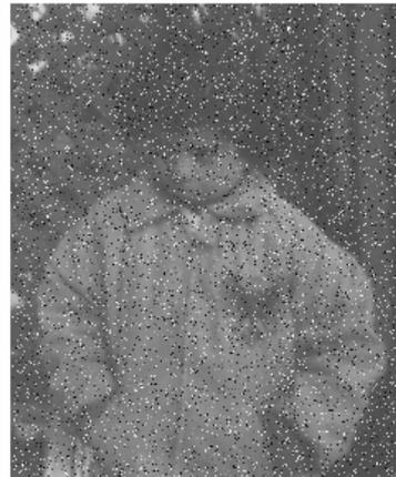
c) Decoded picture with  $MER = 15\text{dB}$
