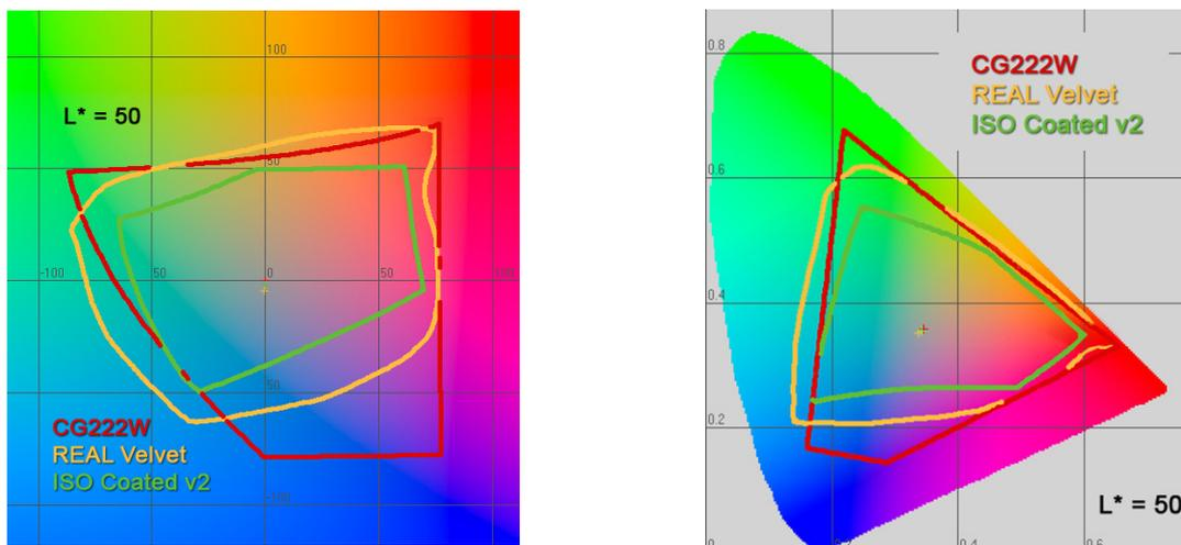
Figure 1: Projection of color gamuts into the ab plane of CIE Lab color space (on the left) and CIE xy chromaticity diagram (on the right)
