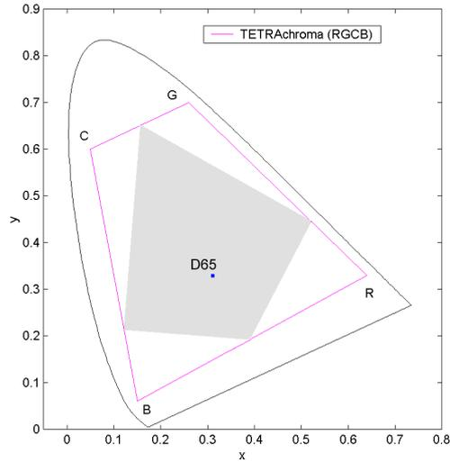
Figure 3: Reproducible area (grey) as a result of minimum norm solution with condition about non-negative elements of control signal  $\mathbf{c}$
