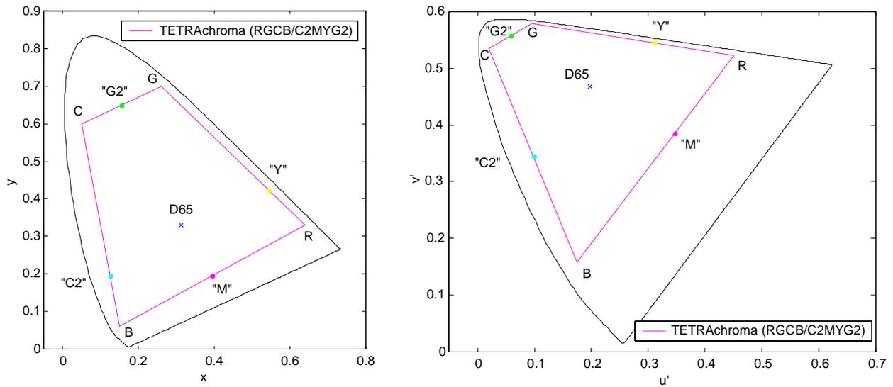
Figure 4: Primaries of Tetra-chroma<sup>4</sup> Display Unit in CIE xy (left) and CIE u'v' (right) chromaticity diagram
