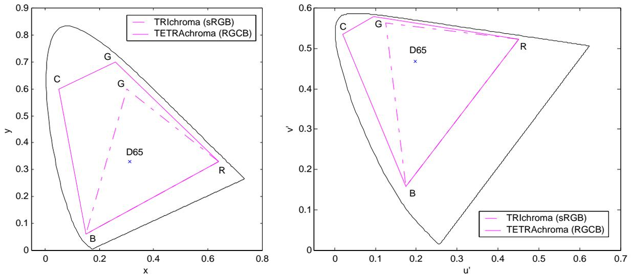
Figure 2: Conventional sRGB and proposed RGCB color gamut in CIE xy (left) and CIE u'v' (right) chromaticity diagram
