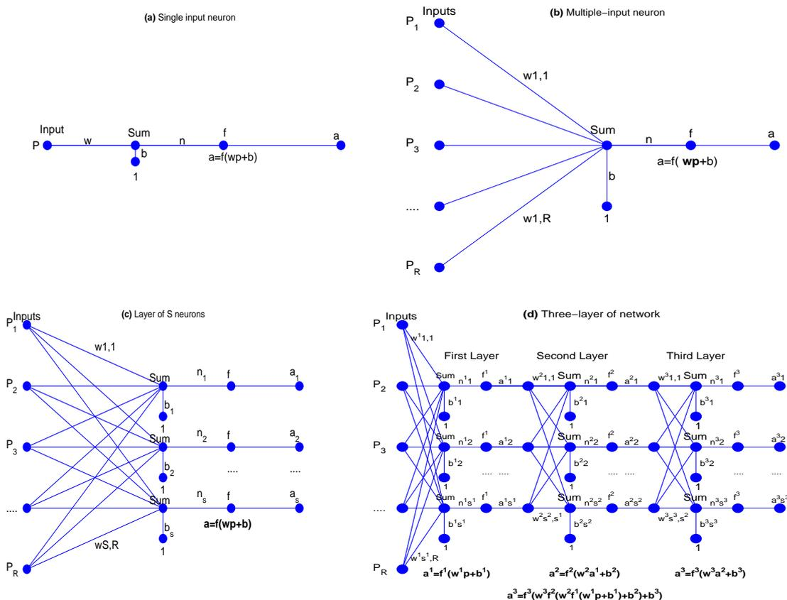
Figure 2: Different structures of neural networks presenting (a) a single-input neuron with a bias, (b) a multiple-input neuron with biases, (c) a layer of neurons, and (d) multiple layers of neurons
