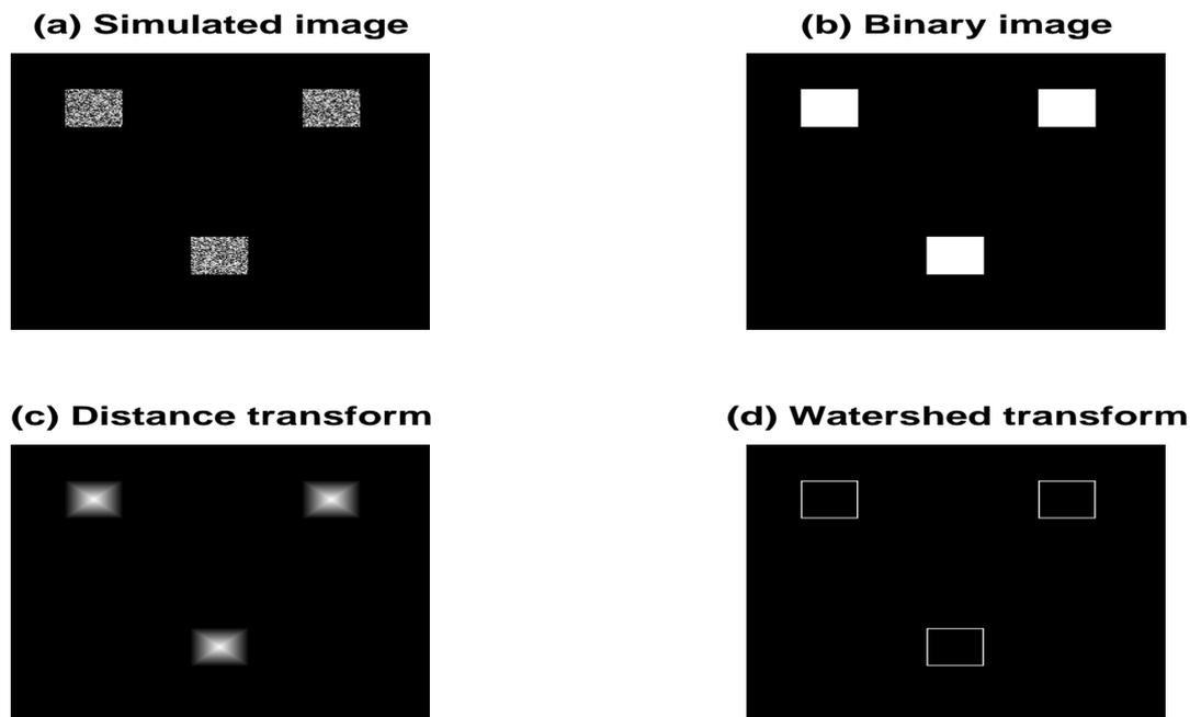
Figure 3: Process of segmentation including (a) simulated gray-scale image, (b) its conversion to the binary image, (c) results of the evaluation of the distance transform of complementary binary image, and (d) watershed transform
