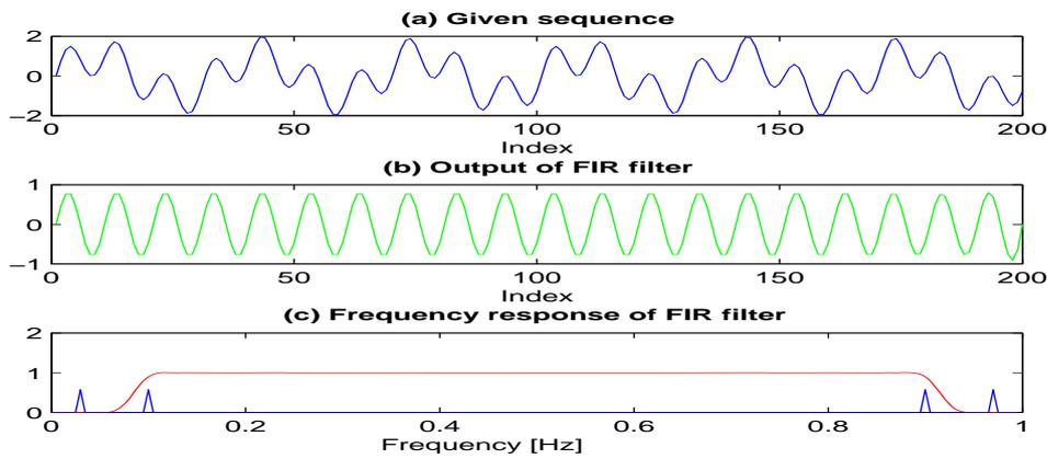
Figure 1: FIR filtering (a) the given simulated sequence formed by the sum of two harmonic functions, (b) result of its processing by the FIR filter of order  $M = 60$ , and (c) frequency spectrum of the given sequence together with the frequency response of the FIR filter
