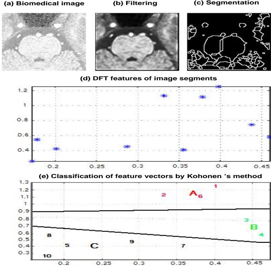
Figure 4: Processing stages of a selected biomedical image presenting (a) the given image, (b) results of its median filtering, (c) evaluation of the Watershed transform, (d) image segments DFT features plot, and (e) results of classification using artificial neural networks by the Kohonen's learning rule with class boundaries.
