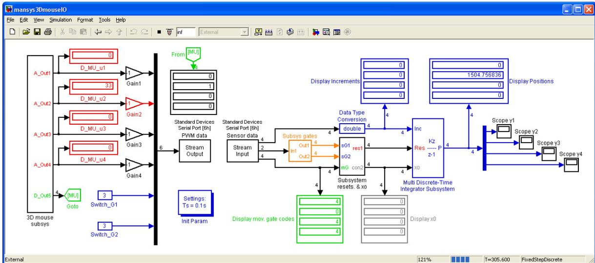
Figure 8: Screenshot of the real-time running Simulink model for simple manual control
