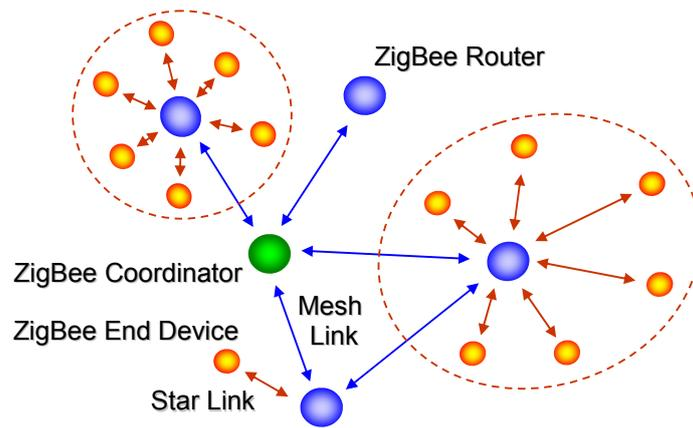
Figure 2: ZigBee network model (network topology)
