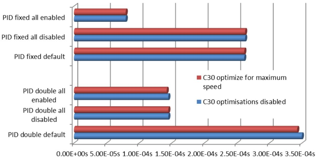
Figure 9: Computing times for C-code generated from the Simulink with default, all optimisations enabled and disabled translated to CPU instructions with different C30 settings.
