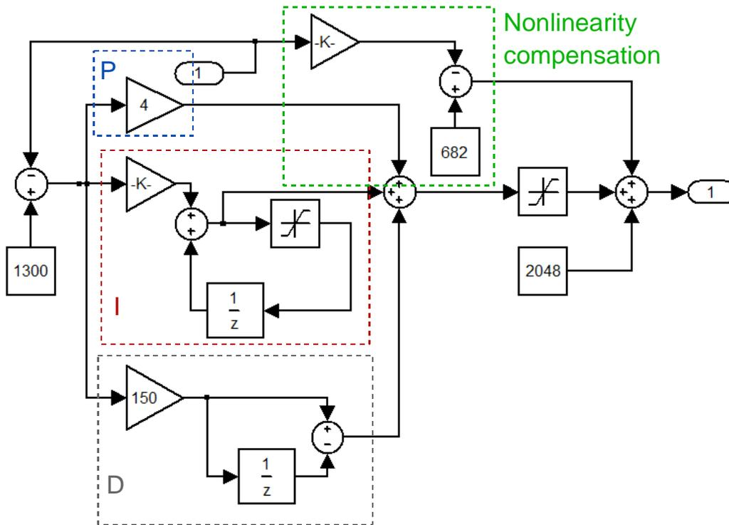
Figure 6: Simulink PID controller scheme.
