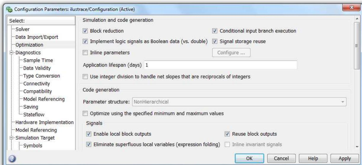
Figure 4: Dialog for changing parameters for the Matlab code generation process.
