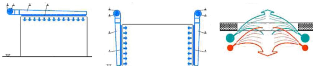
*Fig. 1: Options of installation and the principle of air curtain*
