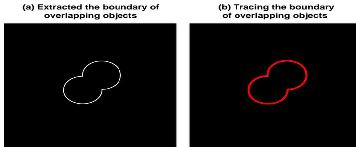
Figure 8: Processing of (a) extracted boundary of overlapping objects, (b) tracing the extracted boundary
