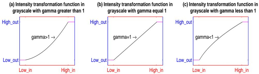
Figure 2: The presentation of intensity transformation functions in the grayscale image with (a) gamma greater than 1, (b) gamma equal 1, (c) gamma less than 1
