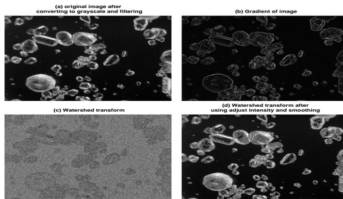
Figure 5: Result of segmentation using gradients image presenting (a) original image after converting to grayscale and filtering, (b) its gradient after application of Sobel filter on microscopic crystal image, (c) watershed transform associated with over-segmented image, (d) result of repeated after intensity adjustment and gradient image smoothing
