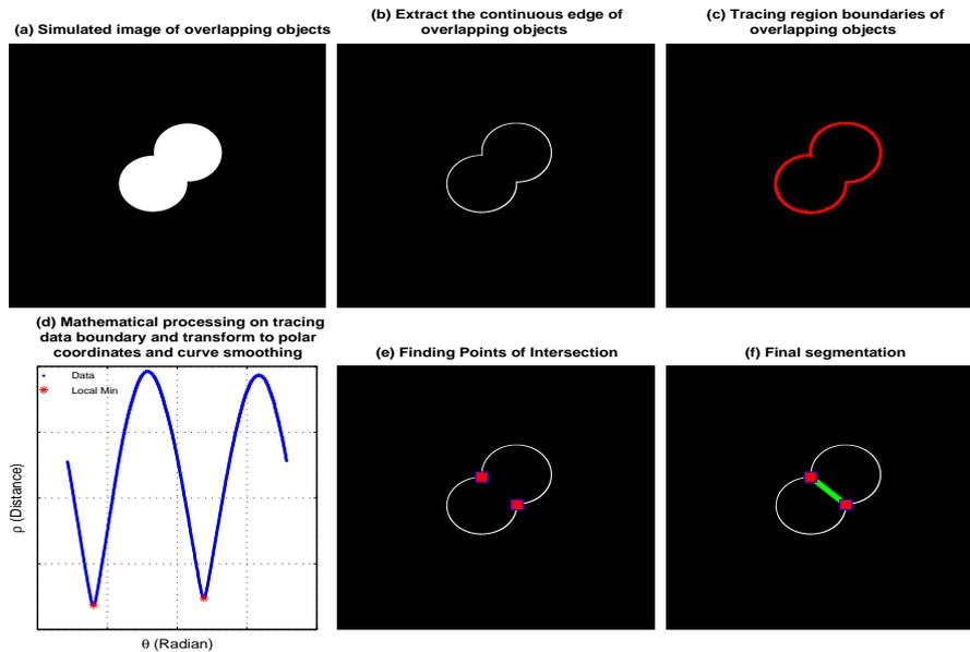
Figure 12: Processing of (a) simulated image (512x512) of overlapping objects, (b) extracting the edge of overlapping objects in a binary image, (c) tracing the edge of overlapping objects, (d) mathematical processing on tracing data boundary and transform to polar coordinates and curve smoothing, (e) identifying the intersection points, (f) the result of final segmentation
