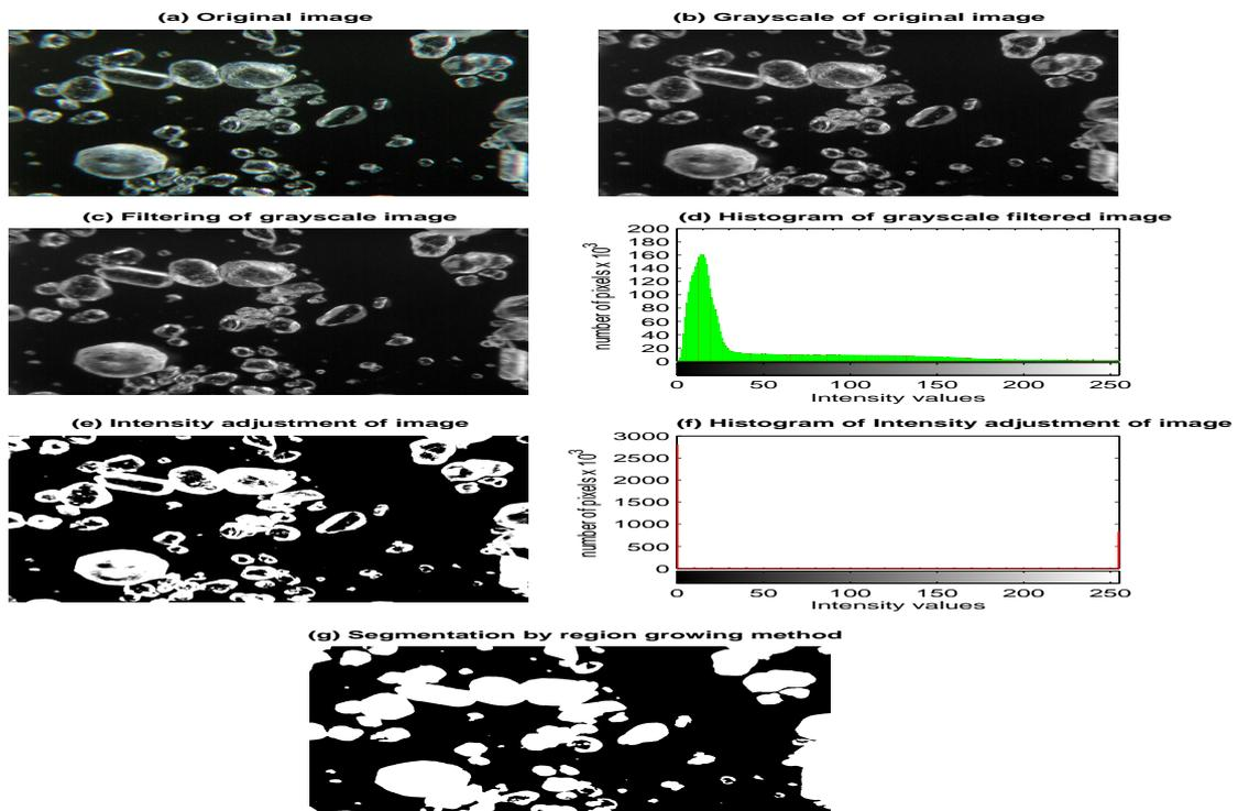
Figure 6: Processing of (a) microscopic crystal image presenting, (b) conversion to grayscale image, (c) filtering of grayscale image, (d) histogram of denosing of grayscale image, (e) intensity adjustment of grayscale image, (f) histogram of intensity adjustment of grayscale image, (g) result of image segmentation by region growing method
