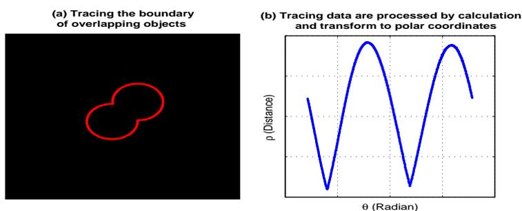
Figure 9: Processing of (a) tracing the boundary of overlapping objects, (b) mathematical processing on tracing data and transform to polar coordinates
