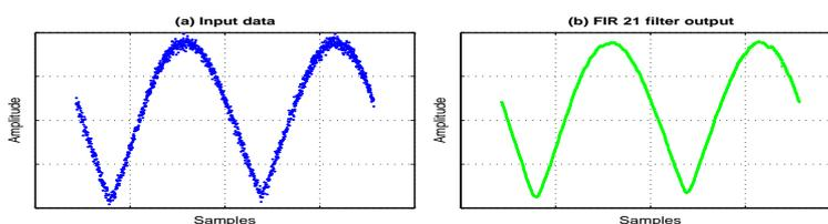
Figure 10: Processing of (a) input sample data and, (b) application moving average filter (order-21) on input data
