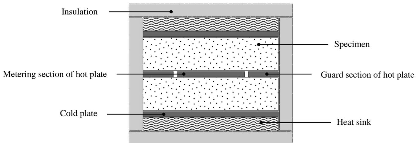
Figure 1 Scheme of double sided GHP apparatus
