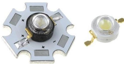
Fig. 1. Display of power LED diode with heat sink and without it
