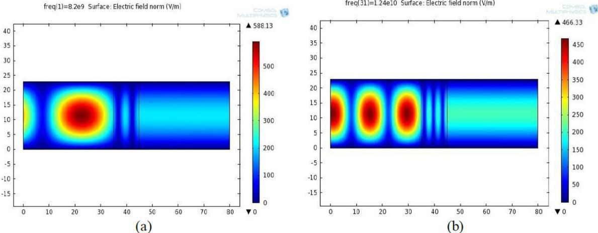
Figure 3: The calculated electric field distribution in the 2D case at 8.2 GHz (a) and 12.4 GHz (b). The DUT is just the jaw (pulp and bone, with  $\epsilon_r=12$ )
