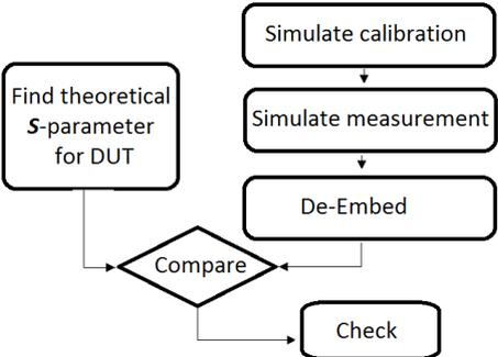
Figure 4: Flow chart to analyse the precision of the 3D EM waveguide simulations
