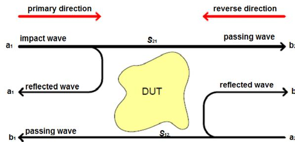
Figure 1: Graphical representation of EM wave distribution in the microwave frequency network (DUT – Testing device)
