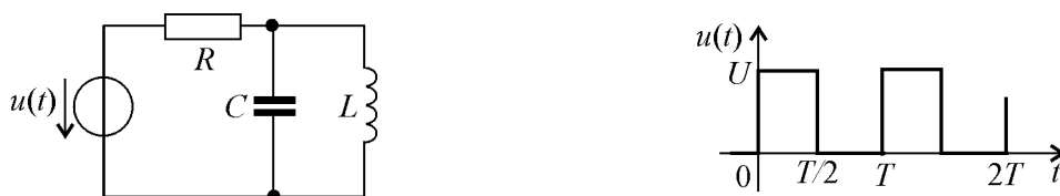
Figure 1: The second-order circuit (left) and the input voltage signal expressed in graphical form (right)
