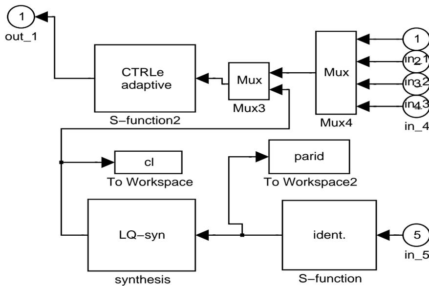
Figure 6: Internal scheme of adaptive controller (unmasked ungrouped)
