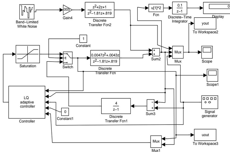
Figure 5: Typical Simulink scheme of adaptive controller
